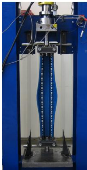
Fig. 10 Distortional buckling of an upright
