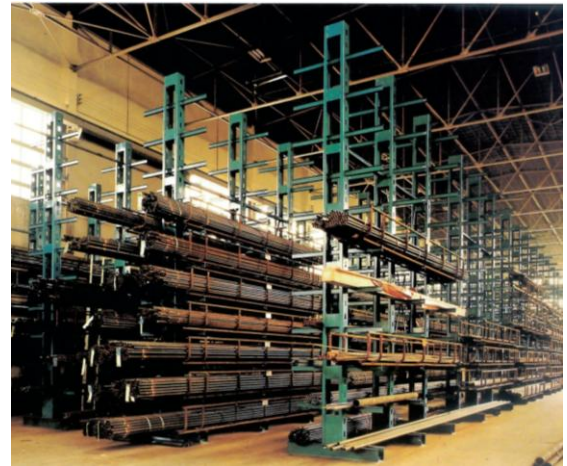
Fig. 4 Example of a cantilever racking
