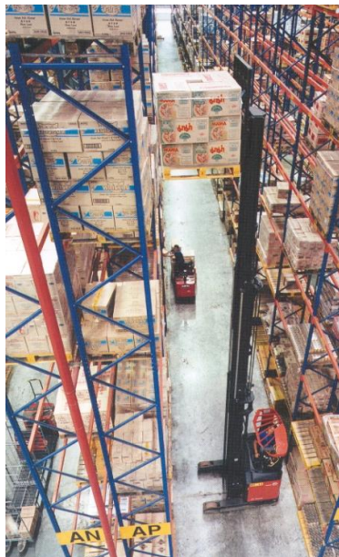
Fig. 1 Pallet rack operated by a reach truck (up to appr. 12,5 m)
