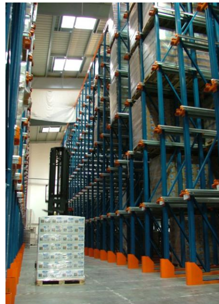
Fig. 2 Drive-in racking operated by a reach truck with side shift
