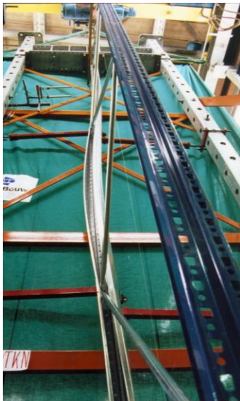
Fig. 9 Torsional buckling of an upright (left sided)
